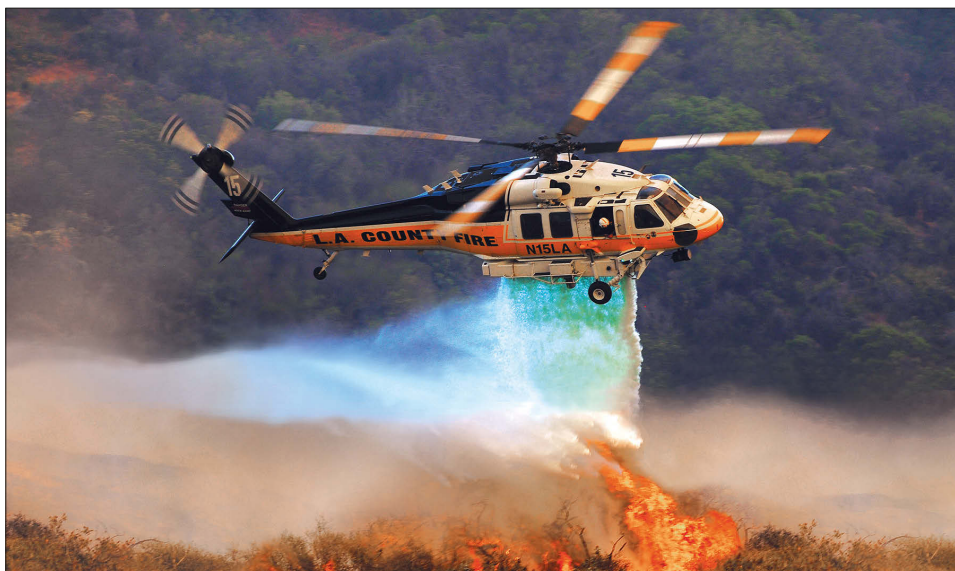
An Isolair system being used from a Sikorsky Firehawk. (Photo: Isolair Helicopter Systems)
