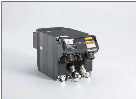
The AN/ARC-210 is a software-programmable V/UHF radio system. (Photo: Collins Aerospace)
