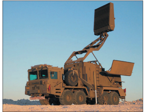
The ESR 220 is a rapid-deployment battlefield local warning radar system which provides low-altitude target detection. (Photo: RRS)
