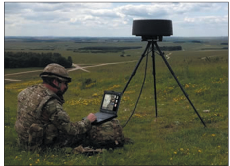
Kelvin Hughes' SharpEye SxV is an X-band lightweight ground surveillance radar. (Photo: Kelvin Hughes)
