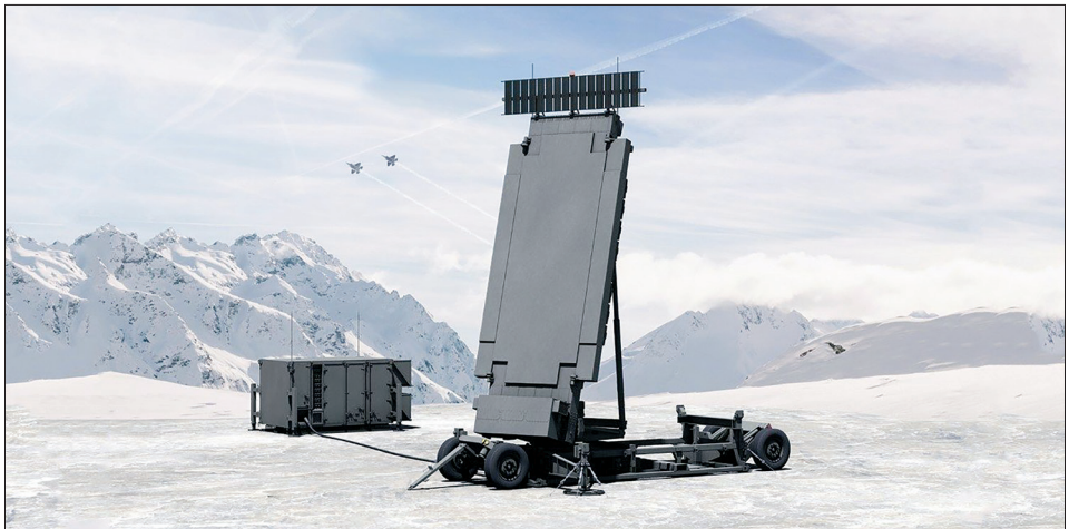
TPY-4 is a multi-mission, ground-based radar for air defence surveillance that can operate in contested electromagnetic environments and provides warfighters the ability to detect and track current and emerging threats. (Image: Lockheed Martin)
