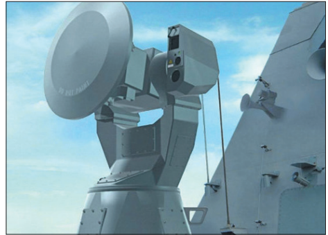
The Oerlikon Seaguard Biax is a naval tracking system with a two-axis multipurpose tracker suitable for all-weather use. (Image: Rheinmetall Air Defence)
