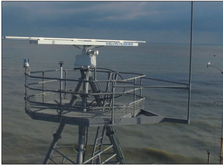
The SBS-900 family of coastal surveillance systems are improved versions of the SBS-800 and provide dual redundancy for the transceiver. (Photo: Kelvin Hughes)
