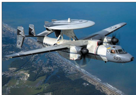
The AN/APS-138 is used on board the seven Northrop Grumman E-2C Hawkeye aircraft operated by the Egyptian Air Force and some of the E-2Cs operated by the USN. (Photo: Lockheed Martin)
