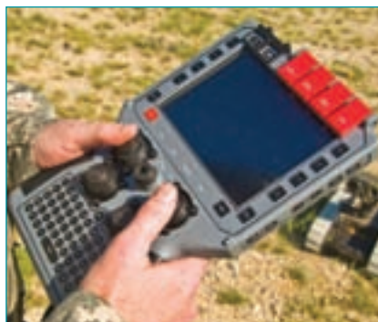
The Common Controller is designed to operate UAVs and UGVs alike. (Photo: Lockheed Martin)
