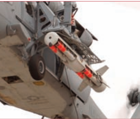
The BAE Systems Archerfish has been designed as a one-shot mine neutralisation system. The company is currently under contract to provide this AUV to the US Navy. (Photo: BAE Systems)
