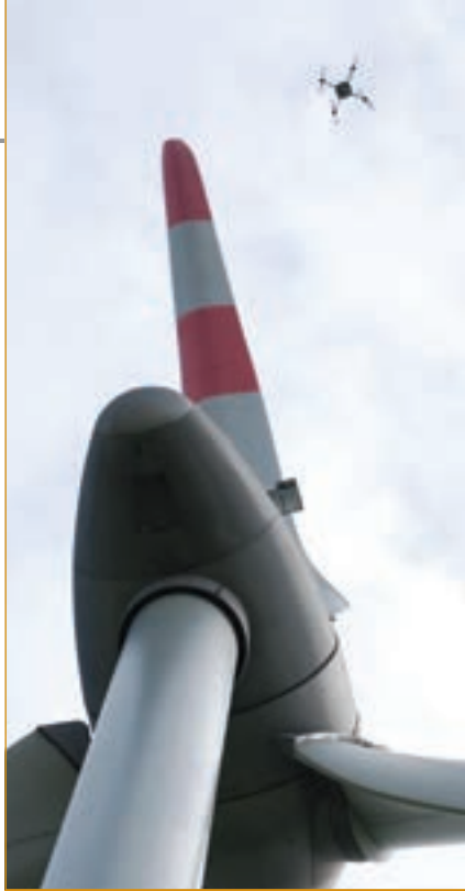
A Sky-Futures-operated Aeryon Scout platform conducts an inspection of a wind turbine. (Photo: Sky-Futures)
