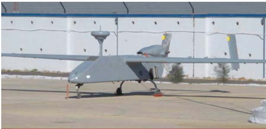
Searcher UAVs can be equipped with EO, COMINT and ESM payloads. (Photo: Indian Navy)
