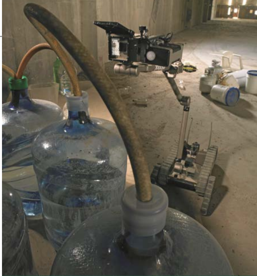
iRobot's 510 PackBot is seeing its role expand to include CBRN missions. (Photo: iRobot)
