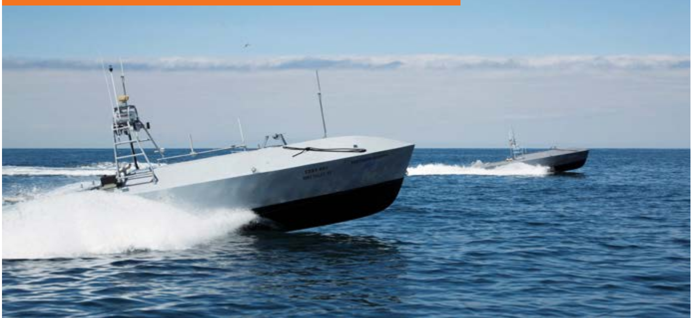
Textron's CUSV has 'sliding autonomy', allowing changes to operator input. (Photo: Textron Systems)
