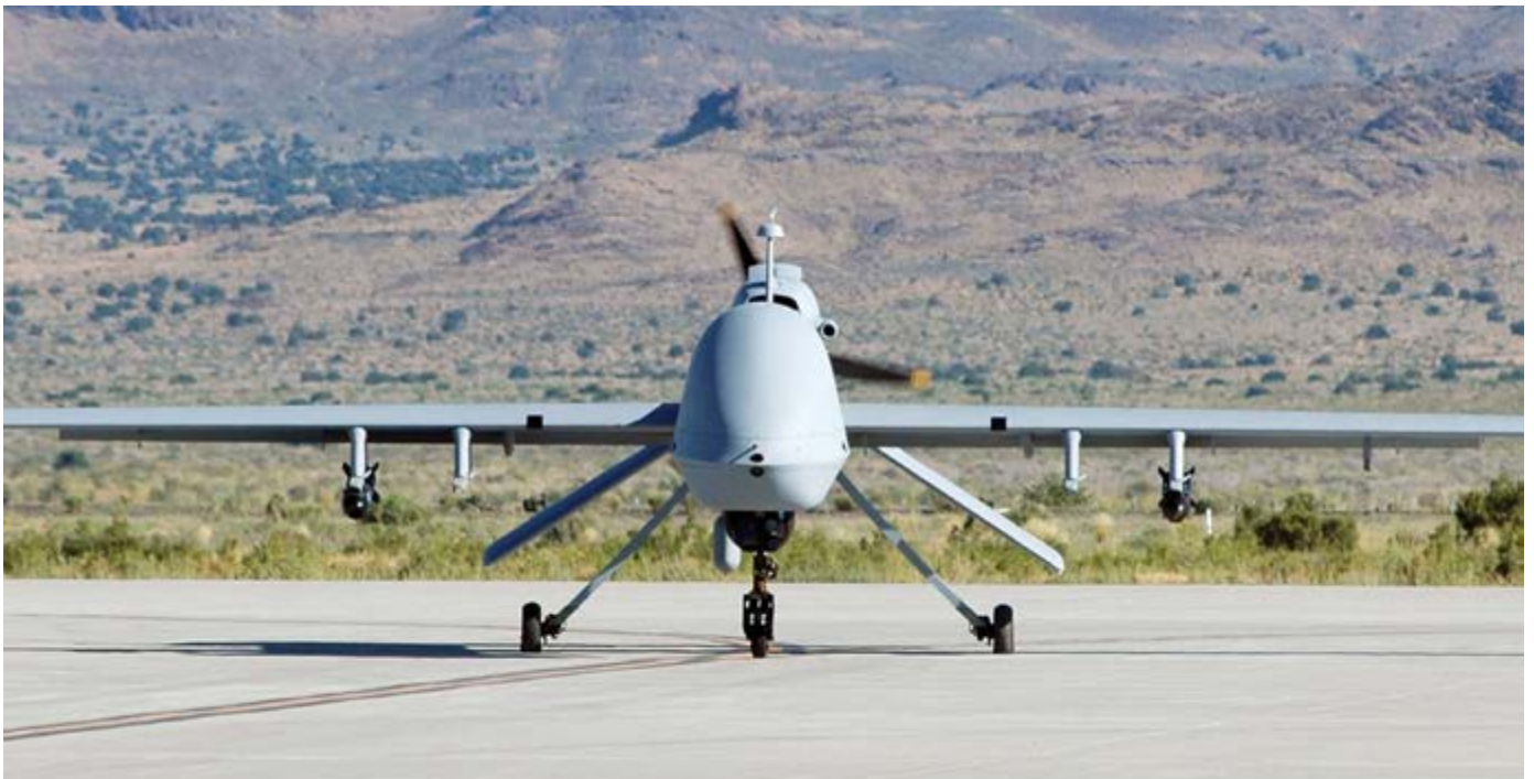
The General Atomics MQ-1C Gray Eagle is equipped with BAE Systems' Tactical SIGINT Payload. (Photo: GA-ASI)
