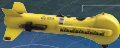
A9 AUV providing stability and accurate navigation for several French Navy programs
